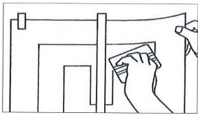
Fold back and squeegee graphic to surface beginning at center of tape and working outward using firm overlapping strokes.
